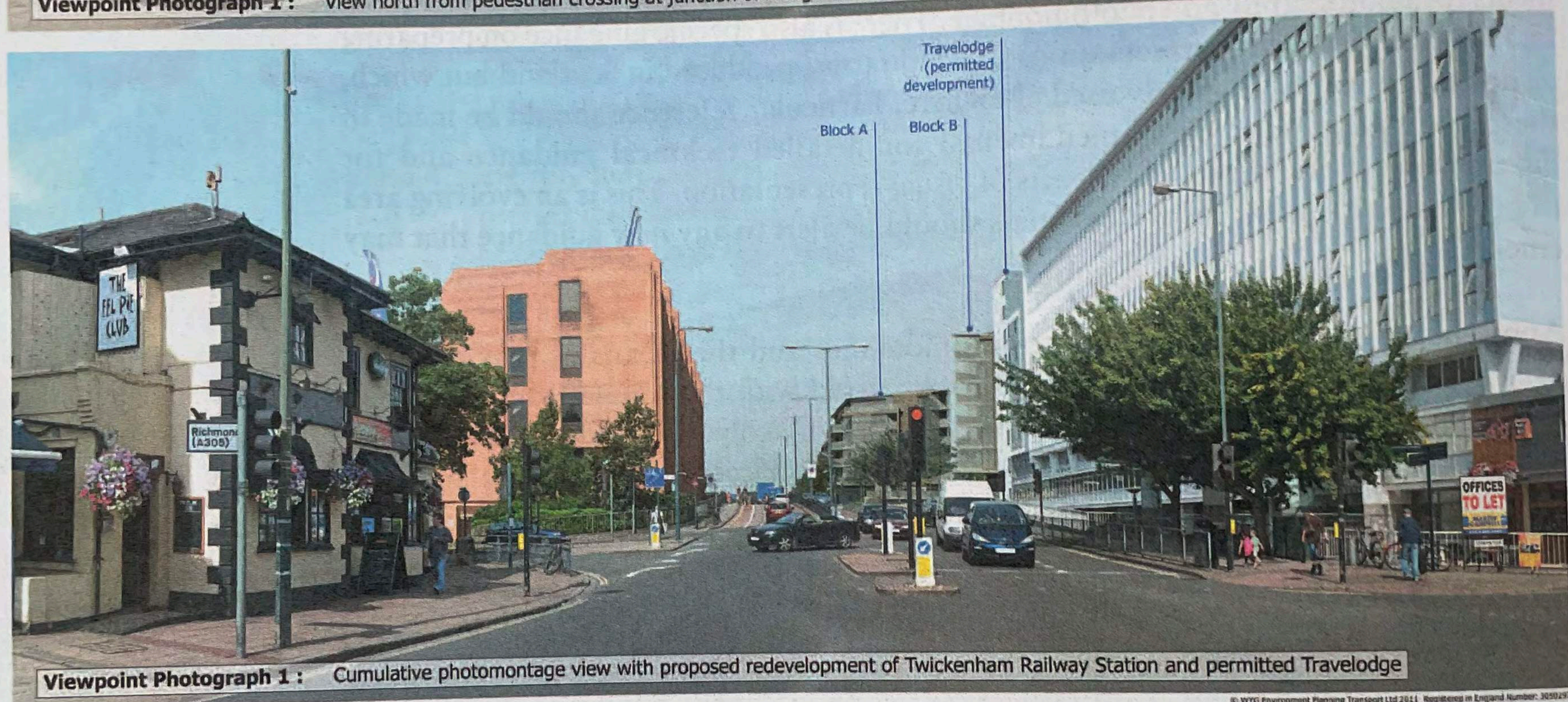
Figure 8.3 Cumulative photomontage of redevelopment at Twickenham Railway Station with other permitted development, a neighbouring hotel extension. Note the aspect ratio of the image to encompass the vertical field of view of the urban context; camera used in portrait orientation
